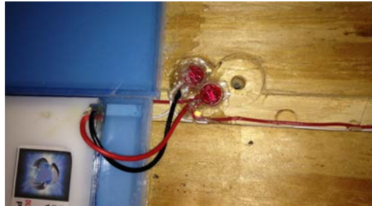
Figure 9 Connector / wires secured with hot glue
